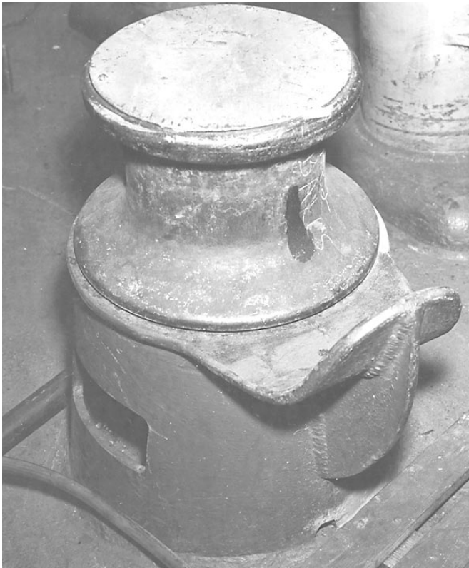
Figure 7-9.—Roller bitt saves line.
